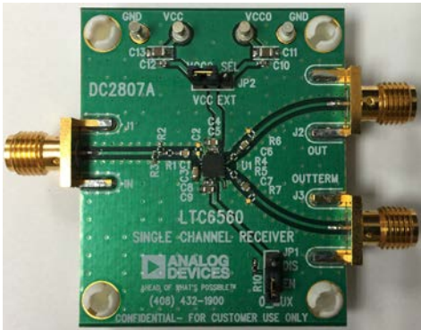
Figure 16. DC2807A Single Channel Electrical Evaluation Board
